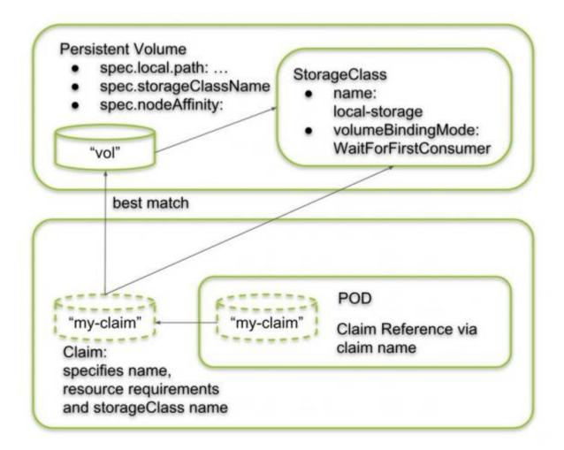
Once a POD is created that references the volume claim by name, a "best match" choice is performed under the restriction that the storage class name matches as well.
